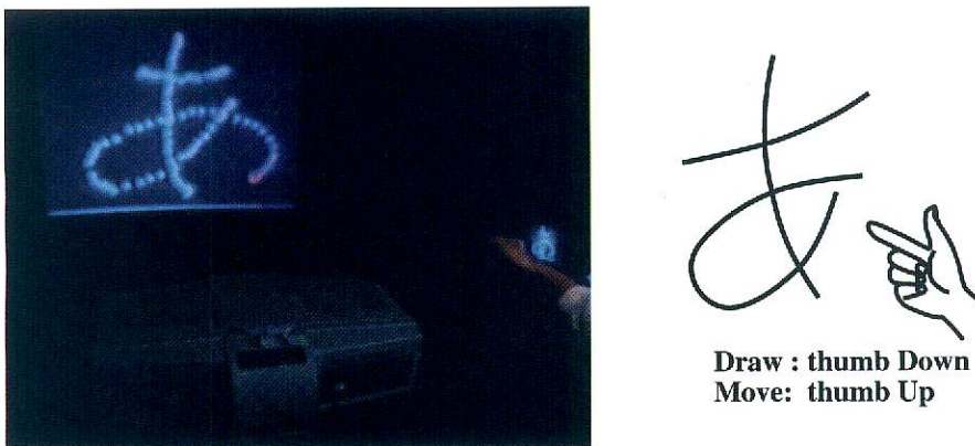
Fig. 16. Drawing characters in space. The system can detect letters and simple figures written in space by finger.
